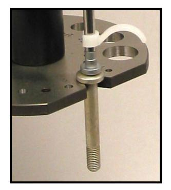
7. <u>Measuring Head Protrusion</u>: To measure a flat head screw's protrusion height rotate the gaging plate so the hole size marking on the plate corresponding to the
