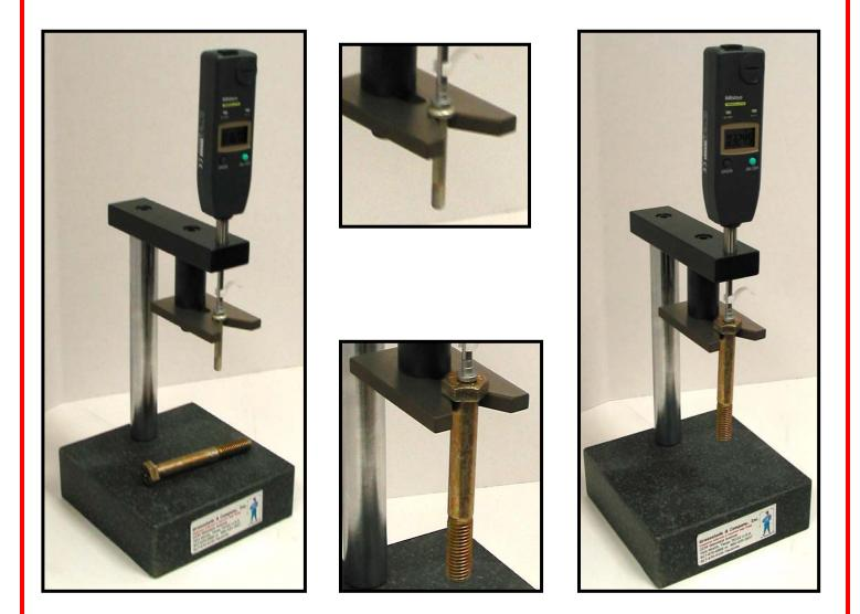
If the user is only interested in measuring head heights this is the gage to select. The "V" arm has an elongated hole so the "V" can be moved toward the back of the gage when measuring large screws and can be moved forward for measuring smaller screws.
