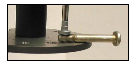
6. <u>Measuring Screw Head Heights:</u> To measure a screw's head height rotate the gaging plate so the indicator foot is resting over the "V" notch in the plate.
