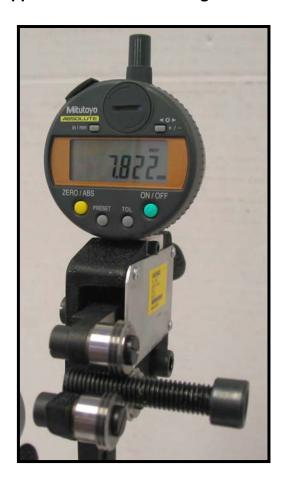
Inspecting the thread's minor diameter
