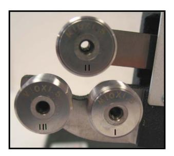
7. With the arm at rest press the pre-set button and the gage is ready to inspect Left Hand threaded product.
