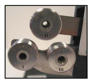
Proper roll mounting for measuring right hand threads
