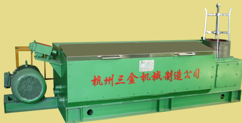
▲ LT15/450重型水箱拉丝机 LT15/450 water tank drawing machine
