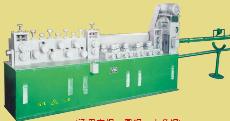
◀ YGT-4/10异型钢调直切断机 YGT-4/10 rebar straightening&cutting machine
