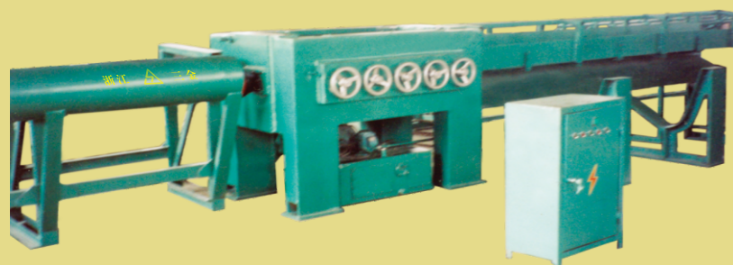
◀ W56-30双曲线辊子型材校直机 W56-30 hyperbola roller section-straightening machine
