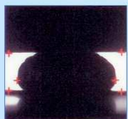
螺頭高度、寬度 Screw-head height, width
