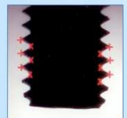
螺牙內外徑 Internal/External Thread Diameter
