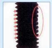
搓牙不良 Bevel Thread/ Deformed Thread
