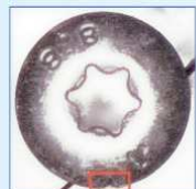
頭上裂痕 Head Crack
