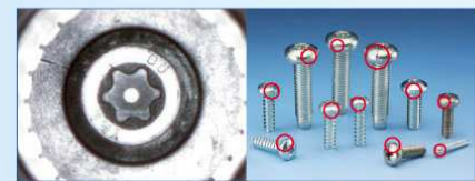
電鍍輪裂螺絲 Zinc Screw of Wheel Crack
