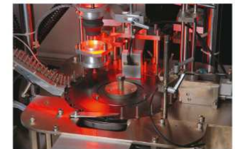
螺牙360°牙傷全檢 Customized Sorting Machine for 360° inspecting thread damage
