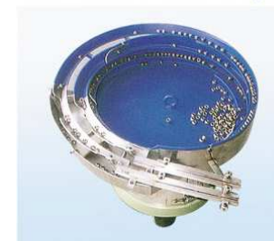
螺帽送料機樣式 Nut Vibration Feeder Sample
