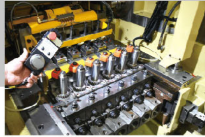
Dial Control Style Slow Jog System 手搖輪慢寸動功能
