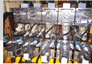
Motorized / digital K.O. length adjustment saves operators a lot of tooling change-over time. (Optional) 人機數位化打模內長度調整 (選配)
