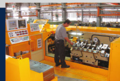
New technical transfer system, Transfer housing lift and turn system, allow operators to set up the transfer easily. (Optional) 新型夾仔台90度旋出外調機構 (選配)
